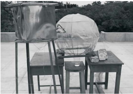
Fig.1. Pictorial view of Spherical Solar Still
