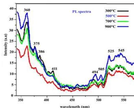
Figure 5. PL spectra at various annealing temperatures
