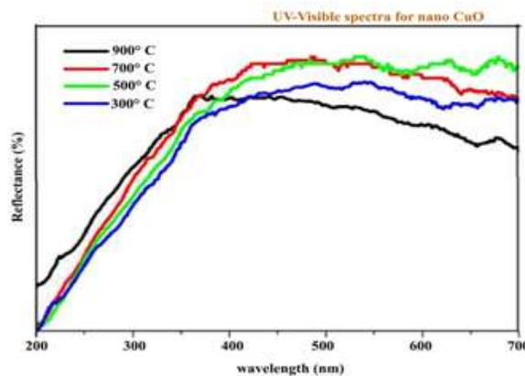
Figure 6. UV-Visible spectra for nano CuO
