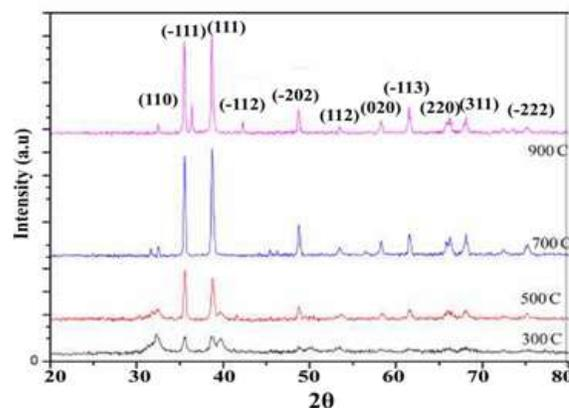
**Figure 1.** The XRD spectral blueprint of prepared sample of  $\text{CuO}$
